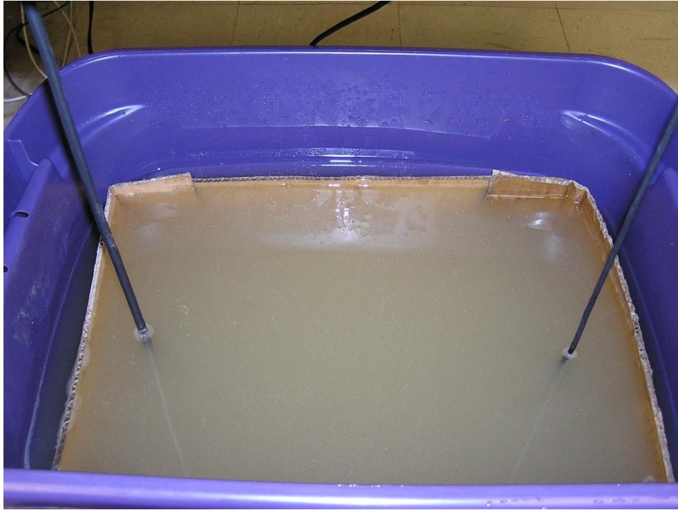
Figure 2-31: Final configuration of underwater channel in office setup. The walls of the tub were lined with cardboard and the bottom was covered with sand to reduce multipath propagation.
