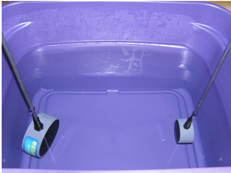
Figure 2-20: Initial configuration of underwater channel in office setup.
