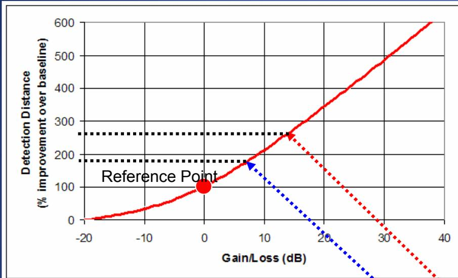
Keeping the other parameters constant, using an array of 6 hydrophones will increase the average gain by 8 dB, resulting in a detection distance 180% greater than the baseline distance.
