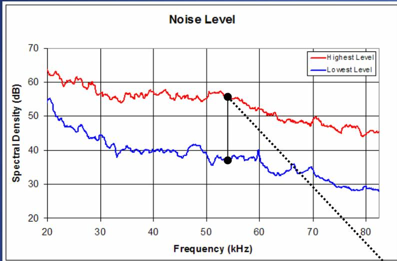
Keeping the other parameters constant, a higher noise level of about 17 dB reduces the overall gain by the same level, resulting in a detection distance of about only 12% of the baseline distance.
